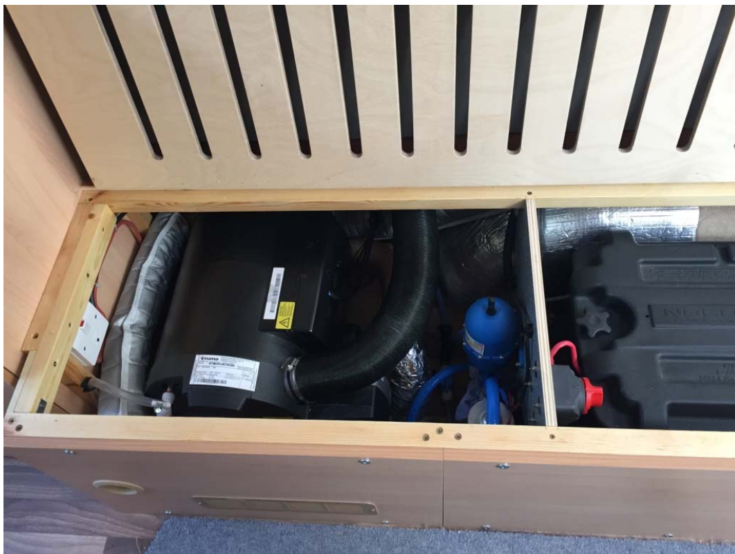
Combination water boiler/ warm air heating system, and water pump - 21/4/2018 -
