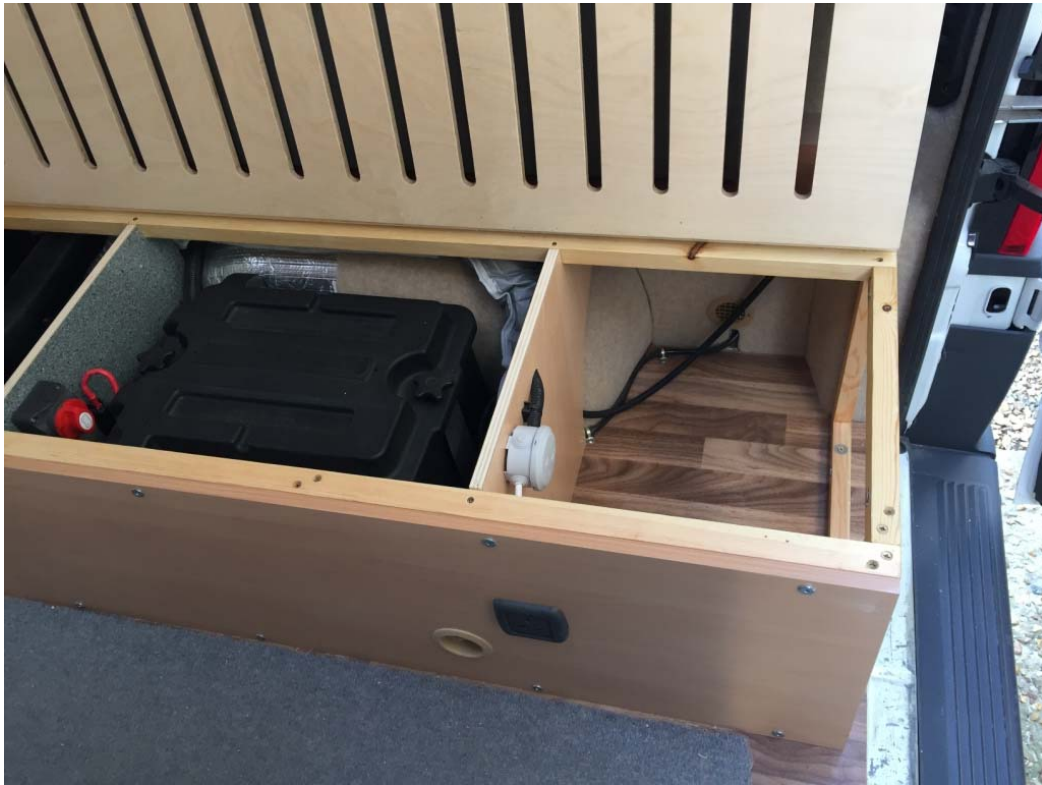
Leisure battery compartment and storage under seat 1 - 21/4/2018 -
