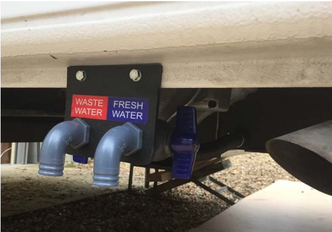
Water system drain taps - 21/4/2018 -
