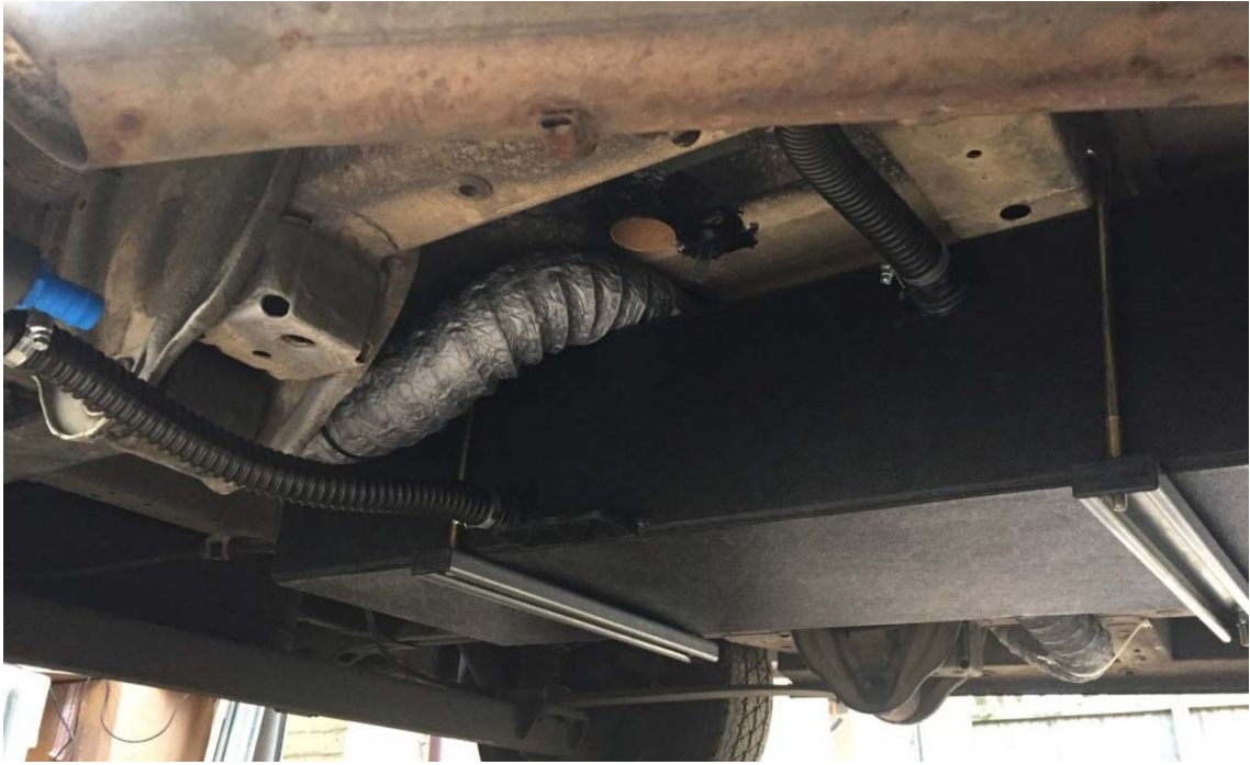
Water tank installation - 21/4/2018 -
