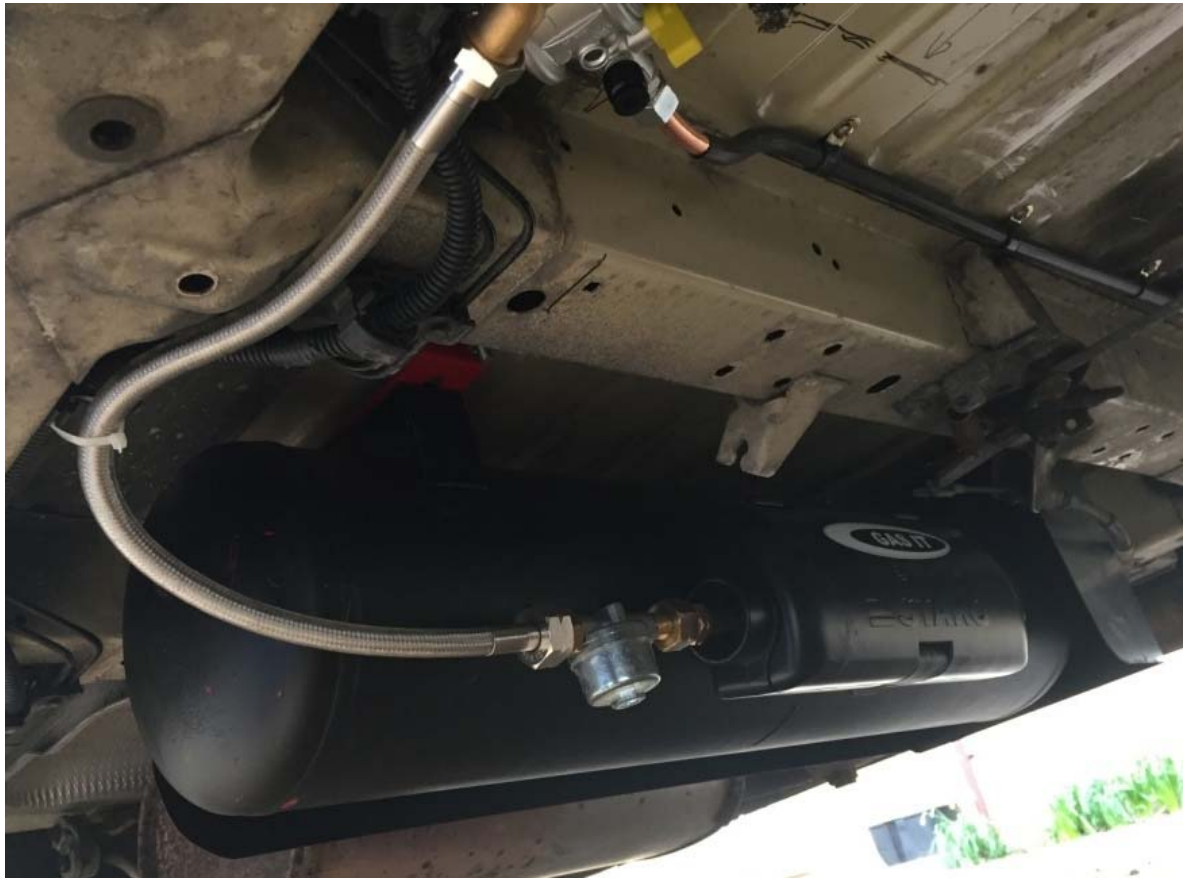
Gas tank installation under van - 21/4/2018 -
