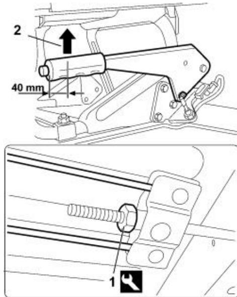
1. Working underneath the vehicle, tighten the adjustment nut to the recommended torque (initial tensioning).
