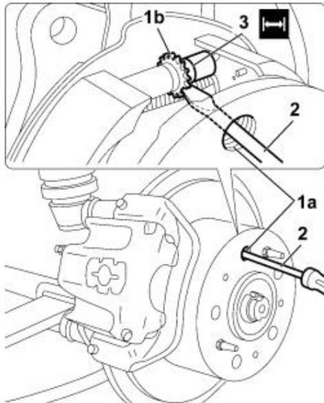
1. Rotate the brake disc until one of the openings (1a) is in line with the toothed pin (1b) for the clearance recovery device.
