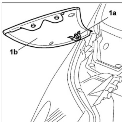
1. Release the retaining pin (1a) and remove the lamp upper moulding (1b) from the vehicle.
