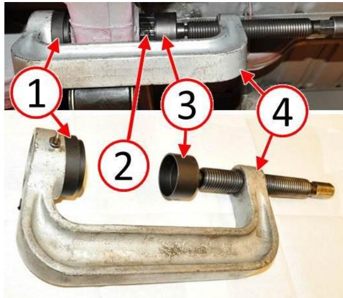
Fig. 12 Press In Inner Bushing
