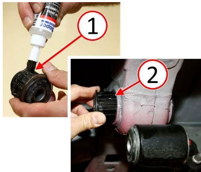
Fig. 10 Install Bushing
