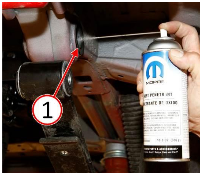
Fig. 7 Lubricate Bushing
