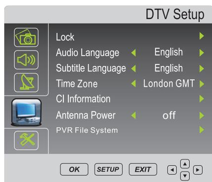
**Antenna Power** – Allows you to turn on/off the antenna power.
