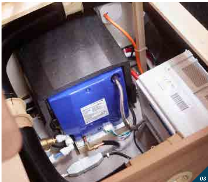
01 Digital control panel 02 Banner leisure battery 03 Whale rapid heat water heater 04 Deep fill bed boxes and underfloor storage
